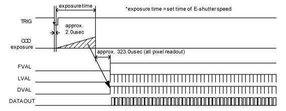
· Pulse Width mode (Trigger Polution:Low Active)
