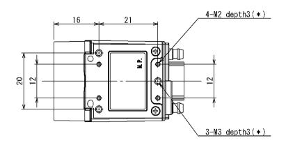
(\*) Depth of screw that can be inserted
