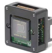
CMOS type : 29×29×16mm (without connector)
