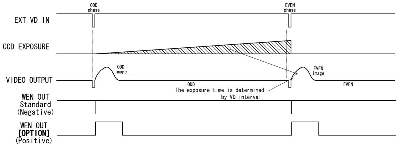
(6) Partial-scan mode selection (CCU bottom-panel DIP SW)
