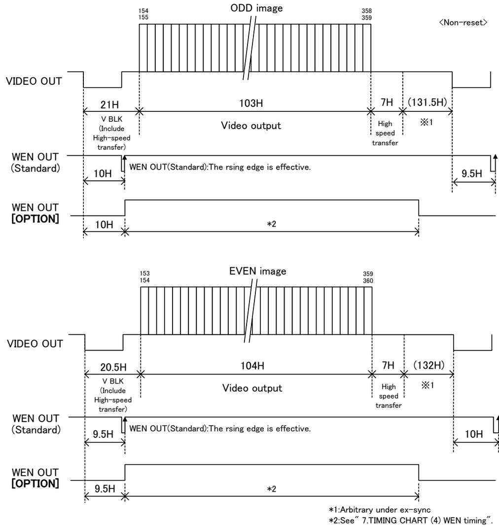
(5-2)1/4 Partial-scan (Rear-panel SW: #8-ON, #9-ON) --- Screen center 1/4 readout
