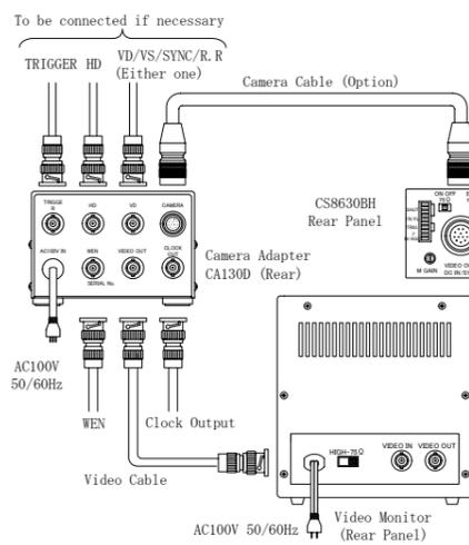
\* Make sure that video output is properly 75-ohm terminated.
