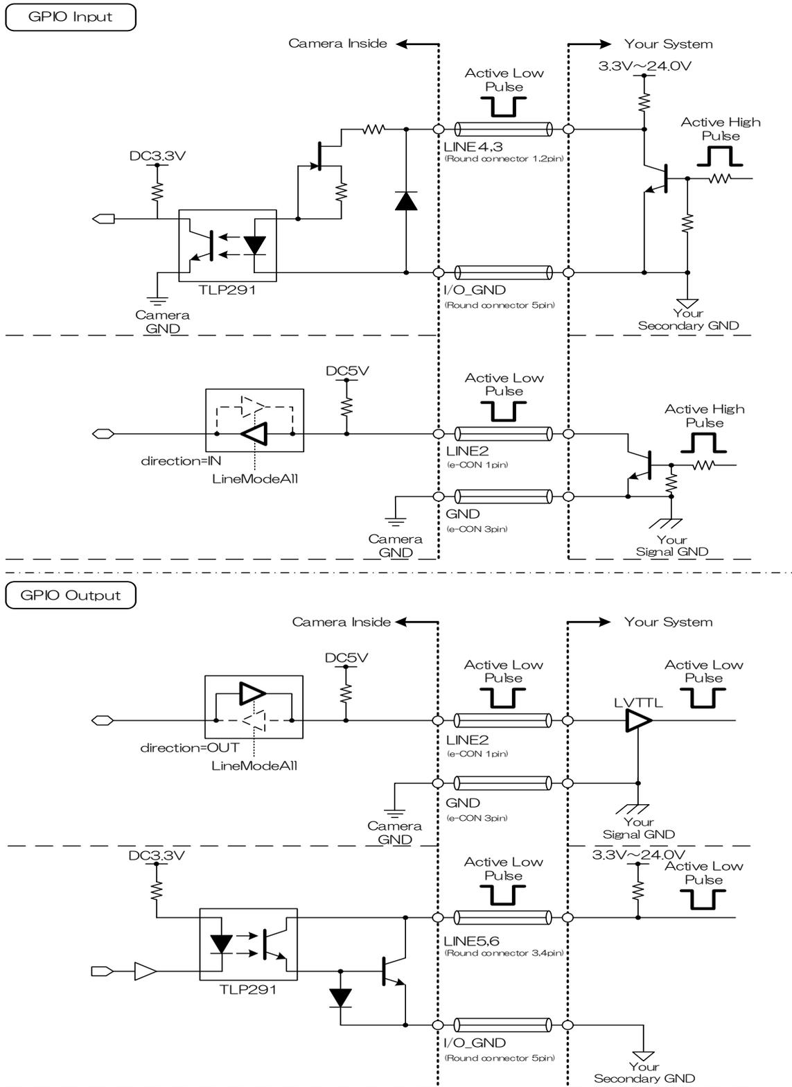
\*Camera GND (e-CON connector Pin 3) and I/O\_GND (Round connector Pin 5) are mutually isolated. It is also possible to connect them to common GND of your system.
