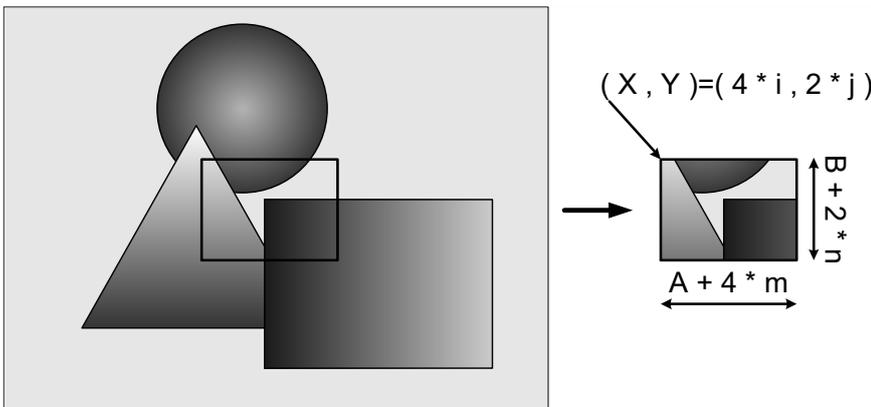
In the scalable mode, camera reads out only necessary area at the normal speed and reads out other area at high speed. The trigger interval can be shorter when the vertical height size is small.
