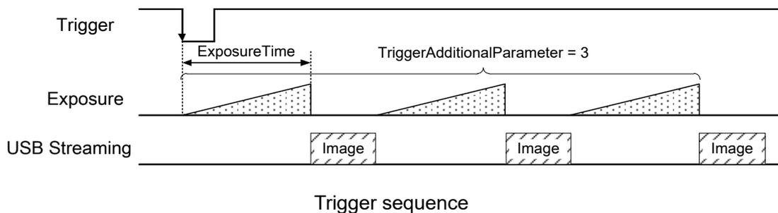
Operation point of HardwareTrigger is at the edge of trigger signal, and active edge polarity is able to change by register setting. And you can add delay time from trigger edge to exposure start by register setting.
