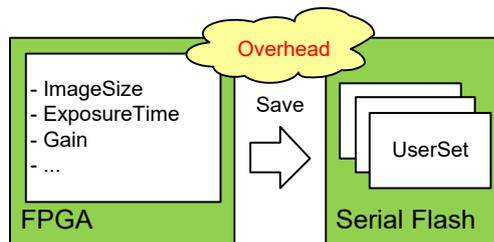
By **UserSetQuickSave**, UserSet is stored to internal RAM. It takes less than **100us** in execution. It can reduce the overhead time of **UserSetSave** greatly. You can also save UserSets to Serial Flash if necessary by **UserSetSave**.
