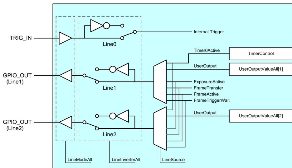
Fig. GPIO internal circuit diagram
