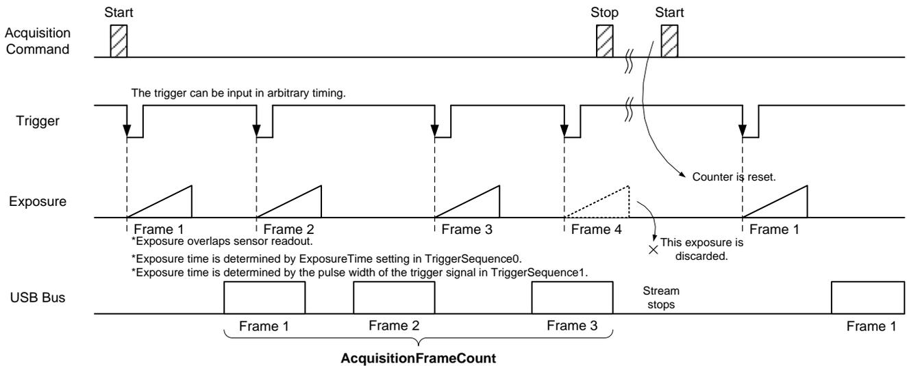
**- Bulk function (TriggerMode = On, TriggerSequence = 6)**
