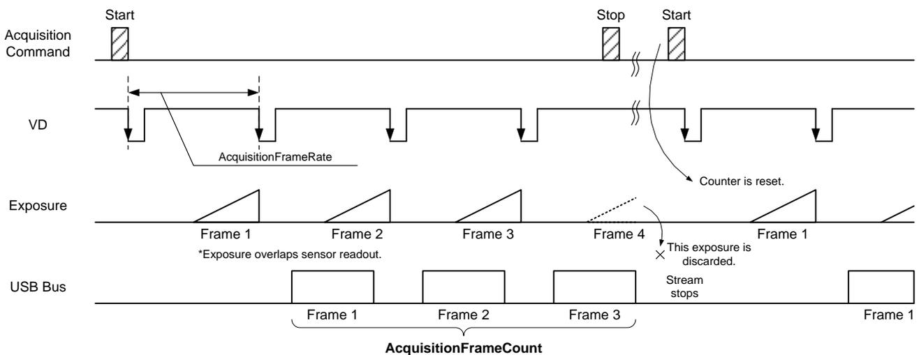
**- MultiFrame function in Random Shutter mode (TriggerMode = On, TriggerSequence = 0 or 1)**
