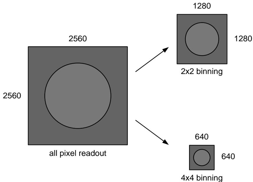
Fig. Binning operation
