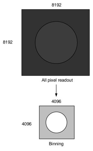
Binning operation (e.g. EX670AMG-X Binning 2x2)
