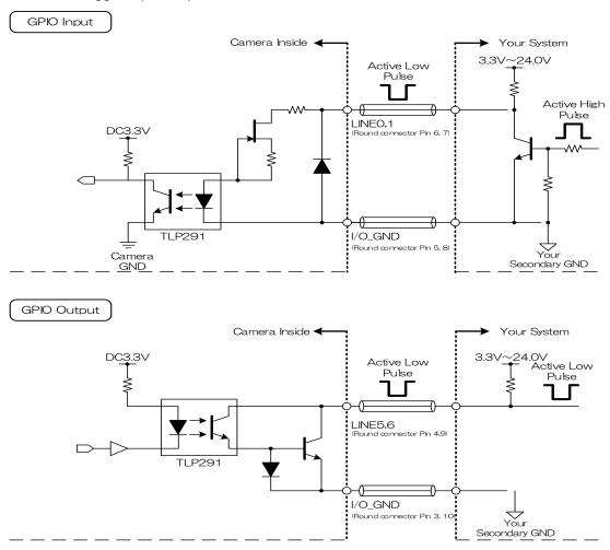
\*Camera GND (e-CON connector Pin 1, 12) and I/O\_GND (Round connector Pin 3, 5, 8 ,10) are mutually isolated. It is also possible to connect them to common GND of your system.
