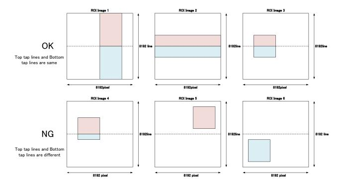
In the scalable mode, camera reads out only necessary area at the normal speed and skips other area at high speed. The trigger interval can be shorter when the vertical height size is small.
