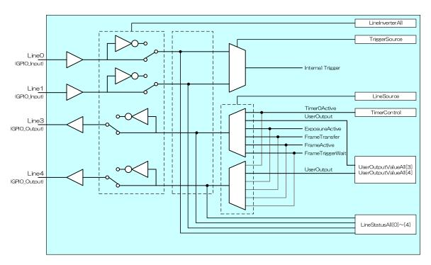
GPIO internal circuit diagram
