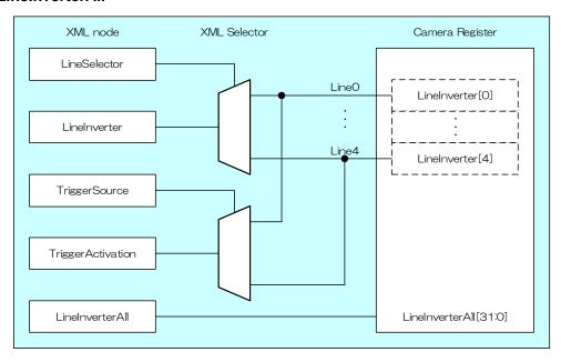
Selects the polarity of each Line signal by 'LineInverterAll'.
