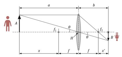
Lateral magnification  $\beta$  is the ratio of image height B against object height A.
